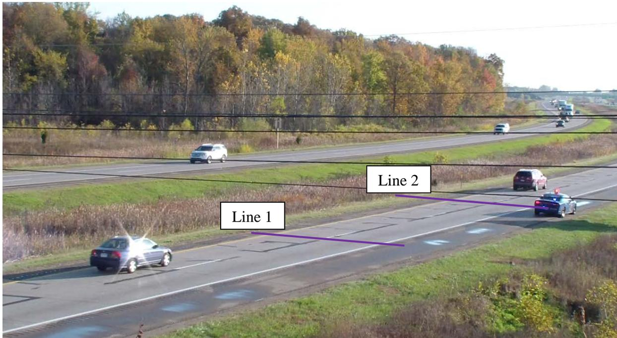
**Figure 19. Reference Line to Measure Vehicle Speed**
